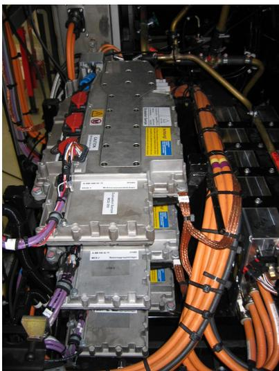
Auxiliary unit inverters for Diesel Hybrid Bus.
